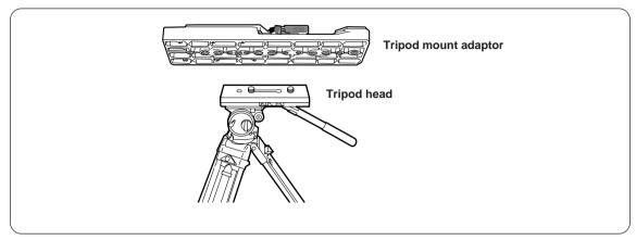
NOTE: Take the center of gravity of the unit and tripod mount adaptor into consideration when selecting the hole for the attachment.
